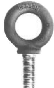
AT 45° lifting angle eye bolts have just 30% of their rated VERTICAL capacity.
