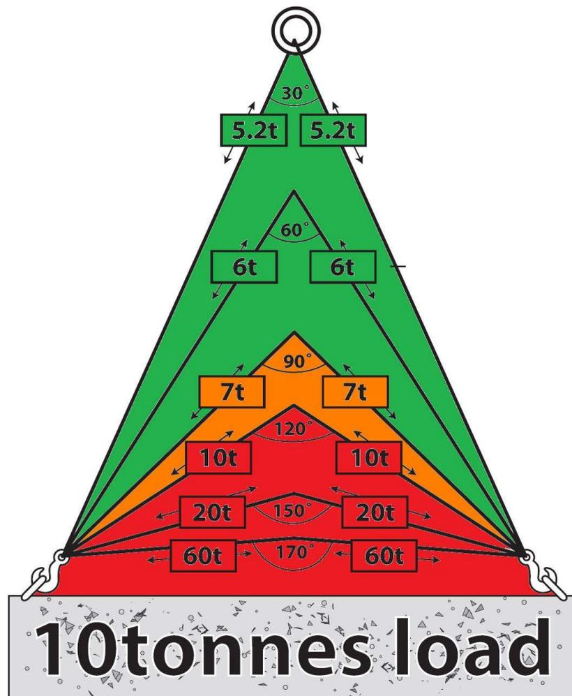
Note: never make sling length shorter than the distance between two anchors
