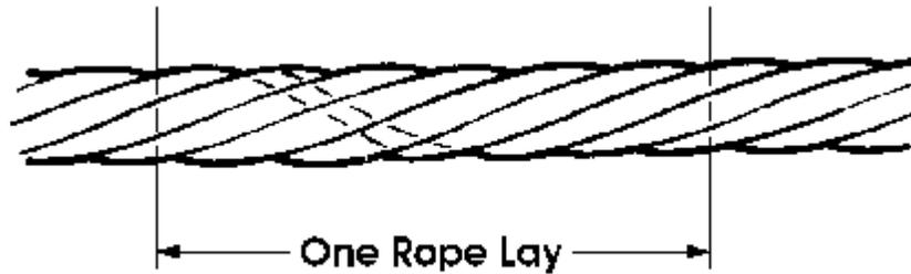
2. *The direction the strands are wound around the core:* Wire rope is referred to as *right lay* or *left lay*. A right lay rope is one in which the strands are wound in a right-hand direction like a conventional screw thread (see figure below). A left lay rope is just the opposite.
