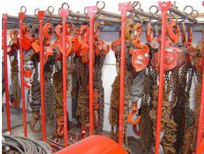
**Chain slings and lever hoists need to be well cared for, and tested if new parts are added**
